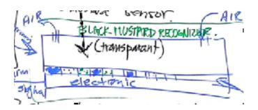
A rough schematic of how this might work is to have a micro analytical array of antibodies with an electronic substrate that draws air through it and detects those places where molecules stuck to the antibodies. Then you could see how antibodies stuck to the electrical substrate and see changes in the responsiveness of the particular parts of the array. This would create a kind of *fingerprint* - an organic chemical sensor.
