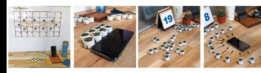
Swarm robots. Ubiquitous robotic interfaces (URI's) – multi-robot interfaces capable of mobility, manipulation, sensing, display, and interaction – were programmed to interact directly with the user and indirectly through surrounding objects. 146
