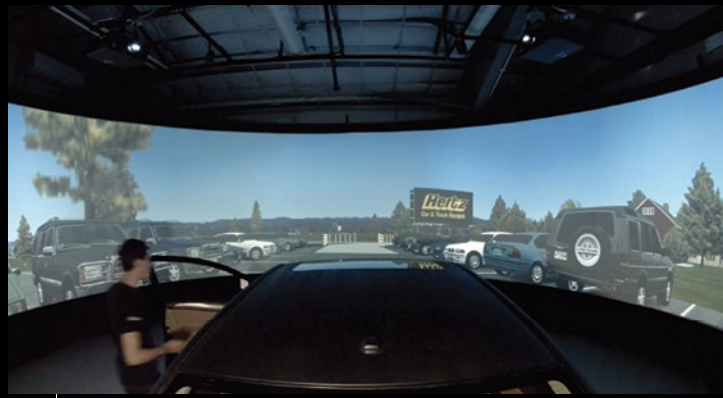
Driving simulator. A life-size surround driving simulator permitted experimenting with drivers' responses to situations and conditions requiring rapid value-based decision making. 163
